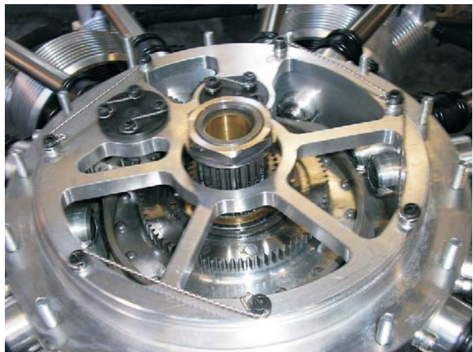
Step 140. This is what the cam plate should look like after safety wiring. TIP. Don't let the safety wire flay about when spinning the pliers, the ends can scratch the nice machined surfaces of the aluminium!
