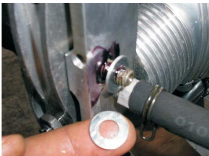
Step 143. Use 10x1 o ring under washer and M8 nyloc. Use 515 as back up sealant. Rocker pin M8 nut must be always pointing to ground. **Temp.** adjust valve screw so about 1/8" arm moment on rocker arm. Tighten rocker pin M8 Nyloc approx. 8'/lbs. Check that rocker is still free and is not pinched between rocker box walls. If its is jammed then slightly back of M8 nyloc nut until free. Not ideal I know, but It works! The 515 thread locks too.
