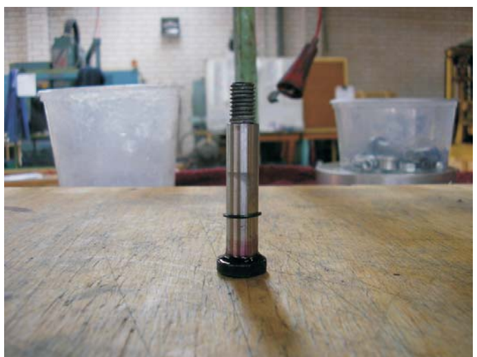
Step 142. Small bead of 515 and O ring positioned on rocker pin ready for installation. NOTE. Position piston on number 1 cyl. at approx. TDC use a blunt rod to feel the piston approach TDC. WARNING: Don't leave blunt rod sit in cylinder free. It will Jam!!! You must draw the feeler rod up with the piston. Wood dowel is safest. Lifters must not be on cam ramps or lobes!
