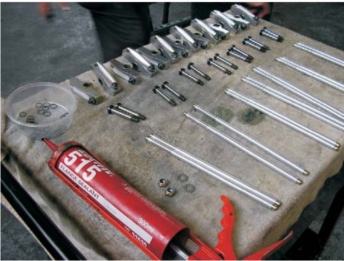
Step 141. Prepare the above. Poke wire thru each end of the push rods to ensure they will transfer oil. Pins should be cleaned of oil. Rockers cleaned with no dirt in roller bearings.
