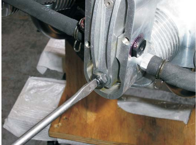
Step 144. Set final valve clearance to smallest perceivable movement of the rocker arm. Zero would be ok. Trust me! With heat The engine grows considerably in operation and the valve clearances open right up. Clean up excess 515. Around rocker pin head and nut. Do the remaining cylinders in a sequential order. You will need to do two rotations between each cylinder to get the piston at approx. TDC with the lifters off the cam lobes i.e. on compression not overlap. NOTE: The cam dot is the centre of valve overlap! Do not set here!
