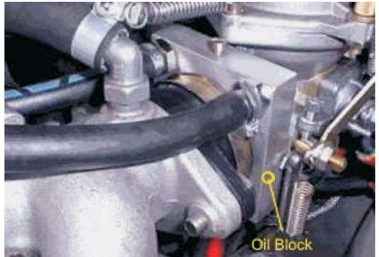
4) In much the same manner as 3) an electric warming element is wrapped around the throat of the Bing carb. For a detailed explanation on how this unit works search for:
